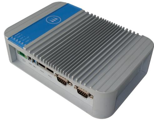
*Eurotech's Multi-service IoT Edge Gateways enable the connectivity between field devices and the Cloud*
