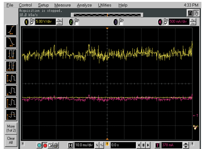
Figure 4- Power Consumption Yellow = power, fuchsia = current, steady Yellow = voltage. MPEG-1 playback, Linux OS is top, WES is bottom. Platform is Catalyst EC.
