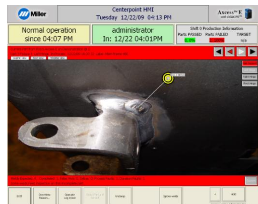
Figure 5: This example output from Insight Centerpoint™ shows the operator interface that guides the operator and monitors each weld for current, voltage, wire feed speed, shielding gas (optional), and duration.
