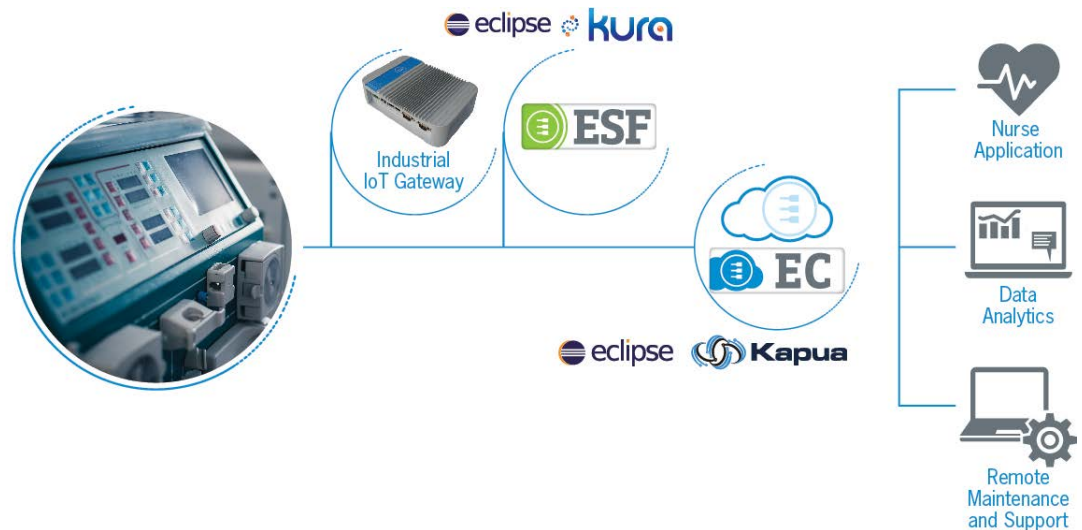
Figure 6. indicates how the two Eclipse building blocks are deployed. ESF (Everyware Software Framework), which is embedded in the gateway, is Eurotech’s commercial, enterprise-ready edition of Eclipse Kura. Everyware Cloud employs a commercial version of Eclipse Kapua, which is the Open Source IoT integration platform.
