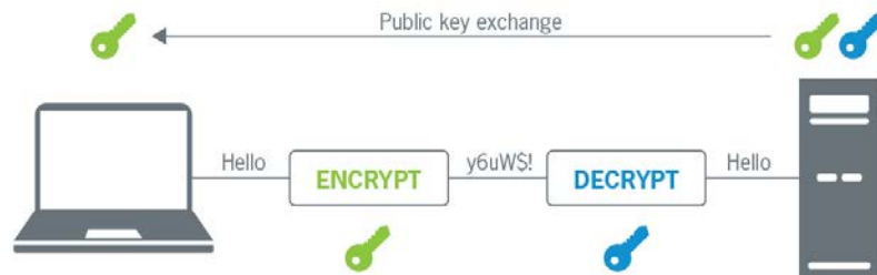
Figure 7. Public-key cryptography uses a separate key for encryption and decryption. Anyone can use the encryption key (public key) to encrypt a message. However, decryption keys (private keys) are secret. This way only the intended receiver can decrypt the message.
