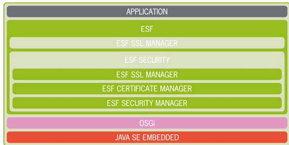
Figure 5. Security mechanisms are an integral component of the Eurotech’s Everyware Software Framework (ESF), which in turn is embedded in the Multi-service IoT Edge Gateway.
