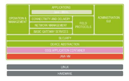
Figure 1. ESF enables wide, deep, seamless integration of applications with the operating system (Linux) and the hardware (devices), while providing full flexibility in terms of programming.
