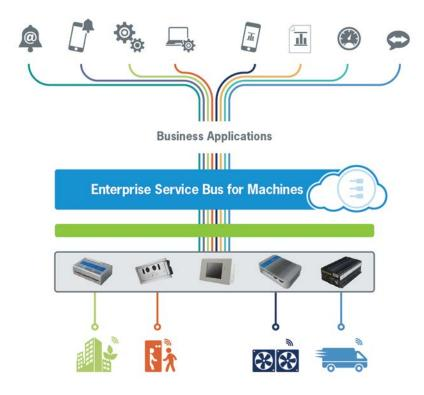
Figure 7. An ESB for Machines allows any relevant enterprise application to interact with any M2M data source. It provides a de facto seamless enterprise extension to an IoT domain.
