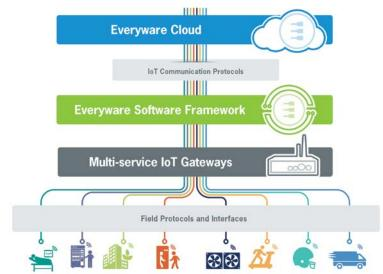
Figure 5. South-facing protocols communicate with the IoT field infrastructure and the north-facing protocols communicate with the IIoT applications infrastructure and the Everyware Cloud. This clearly indicates that the multi-service gateway plays a pivotal, connectivity role in the IoT architecture.
