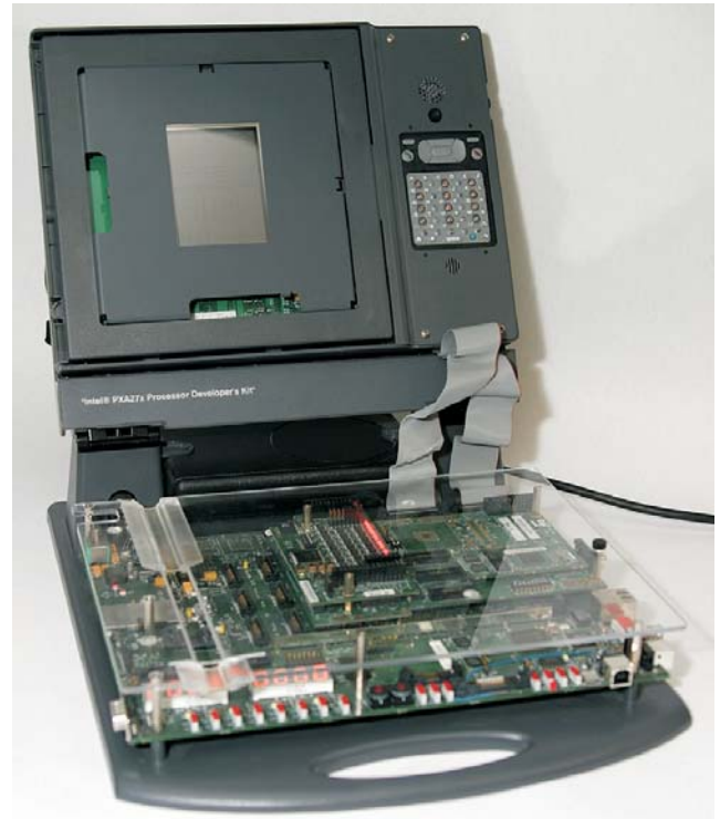
Figure 1- the Intel Mainstone is typical of Silicon supplier dev systems- notice, this was targeted at PDAs and smart phones, but look how many components!!! This is not a refined bill of material.
