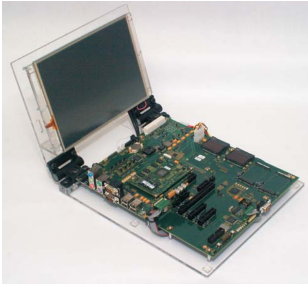
Figure 3- This Development System is based on a ‘module’ and ‘carrier’ board. Software drivers are in place, and the carrier board schematics are available to the customer to facilitate the design of his own product.
