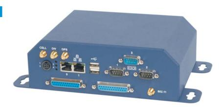
The ZyWAN brings always-on Internet connectivity to any field based device, enabling it to be monitored or relay data back to a central server.
