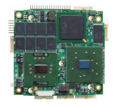
The CPU-1474 is an embedded RoHS compliant board based on two modules: a mezzanine CPU module combined with a PC/104-Plus form factor carrier.
