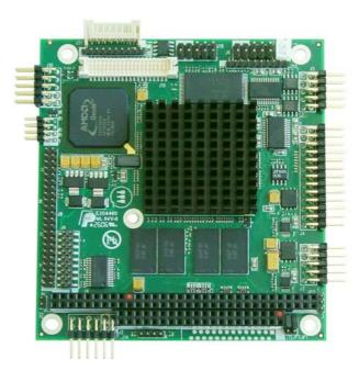
The CPU-1233 is a fully RoHS compliant replacement for the popular CPU-1232 PC/104 module. It now features the AMD™ Geode™ GX466 333MHz Pentium® MMX class processor and is Windows CE® & XPE® and Linux® compatible.
