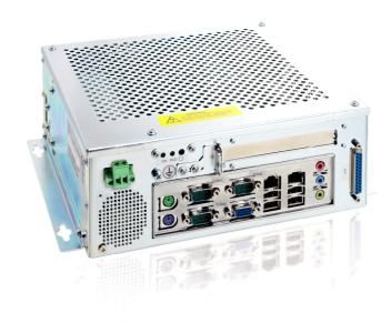
The Eurotech Bx-400F-N270 is a fanless Industrial Box Computer featuring the Intel® Atom $^{\text{TM}}$  N270 1.6 GHz Ultra Low Voltage processor. This feature increases energy efficiency while offering both targeted performance and low power consumption in a highly integrated design. All this while maintaining full Intel® Core $^{\text{TM}}$  micro-architecture instruction set compatibility.
