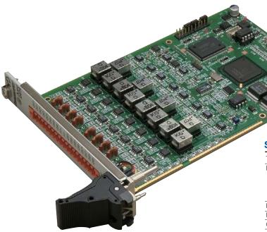
1) 8-channel thermocouple input is possible. As soon as the power is
