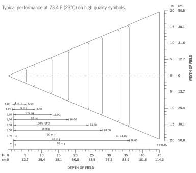
\*Minimum distance determined by symbol length and scan angle
