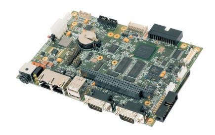
The ZEUS is an ultra-low power EPIC size single board computer based on Marvell's 520MHz PXA270 XScale RISC processor. The PXA270 is an implementation of the ARM compliant, Intel XScale microarchitecture combined with a comprehensive set of integrated peripherals including, a flat panel graphics controller, USB host/client controller, interrupt controller and multiple serial ports. The ZEUS also includes a site for a variety of wireless modems and a GPS receiver.
