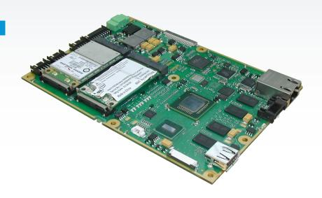
PROTEUS COM Express is a processor module aimed at wired and wireless, net-centric multimedia applications, especially in situations where low power and high performance are required. Using Intel's Hi-K 45nm technology the Intel Atom Z500 series processor delivers the benefits of Intel's x86 architecture in a robust, ultra-small package with exceptional performance-per-watt.
