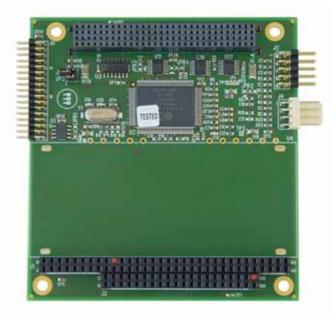
The INT-1462 video frame grabber is a cost-effective, high-performance solution for capturing analog broadcast signals across the PCI bus. Based around the Conexant Fusion<sup>™</sup> 878A video decoder, this compact PC/104-Plus form factor board supports NTSC, PAL, and SECAM video formats at capture resolutions of up to 768x576 pixels and 30 frames per second. It also has the ability to sub-sample, scale, crop, and clip images at various resolutions and frame rates.
