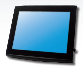
The DuraVIS™ 1500 is a rugged off-the-shelf 15" display featuring a 1024 x 768 XGA LVDS interface. It has been designed for demanding applications that range from vehicle or machine mounted displays to industrial Man-Machine-Interfaces.
