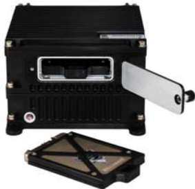
Rear Panel Access to Dual Removable 2.5" SATA SSD Storage
