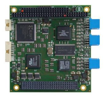
The CTR-1474 is a high performance four channel Video Compressor that accepts all NTSC/PAL standards with auto detection, and benefits by the features and the enhanced quality provided by the JPEG2000 (J2K) image compression standard.
