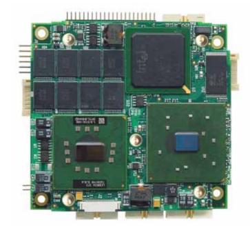
The CPU-1472 is an embedded RoHS compliant board based on two modules: a mezzanine CPU module combined with a PC/104-Plus form factor carrier.
