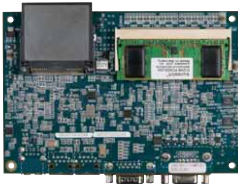
Solder-side: SO-DIMM module and CompactFlash card are optional accessories.
