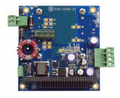
The ACS-5161 is a galvanically-isolated dual-output DC/DC power converter in a PC/104 form factor. Providing up to 100 watts of peak power (minimum 60 watts continuous at extended temps if not structurally heatsinked), the ACS-5161 features a special mechanical design hardened for extreme temperatures and high levels of shock and vibration, making it ideal for aircraft, rail, ship or industrial installations. All the components are securely fixed to the board for shock/vibration resistance.
