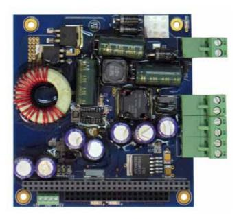
The ACS-5151 vehicle power supply is designed to meet the system design requirements of vehicle, machine, industrial, and mobile installations. It offers resistance to high levels of shock and vibration and has a rugged mechanical design. All heavy components are glued to the board.
