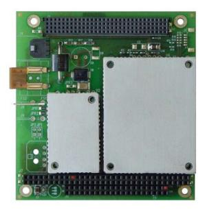
The Eurotech ACS-5125 is a 25W isolated power supply module designed to meet the system requirements of military vehicle, aircraft, machine or vessel installations. The module supplies +5V @ 5A with overload protection and without any de-rating.
