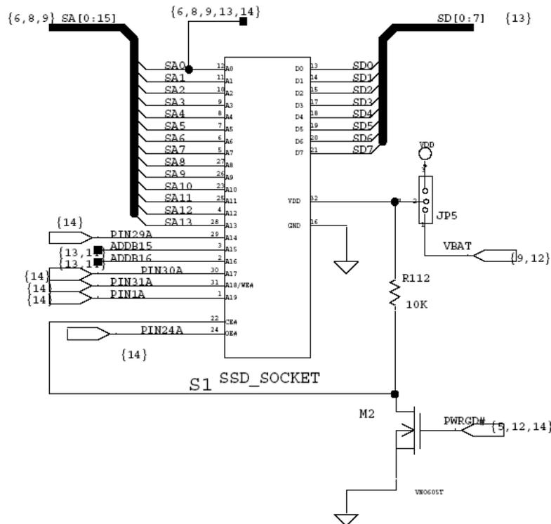
The PWRGD# signal is used on the logic to control the chip selection for static RAM to prevent erroneous writing access into memory during no valid power supply periods when data lines are not stabilized and supply of the SSD Socked is present because it is derived directly from battery.
